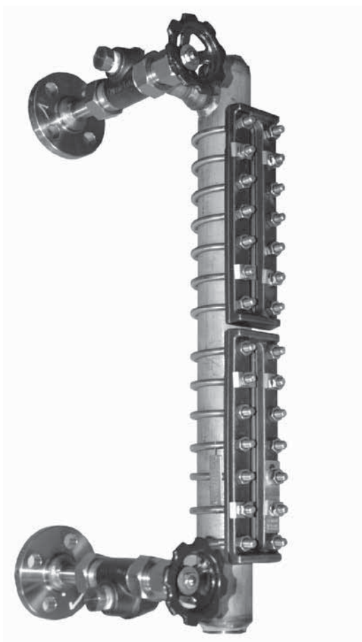
EXAMPLE: 72RL-LC-CH [No. 7 glass, 2 section, reflex, low pressure, side/side connection, large chamber]
